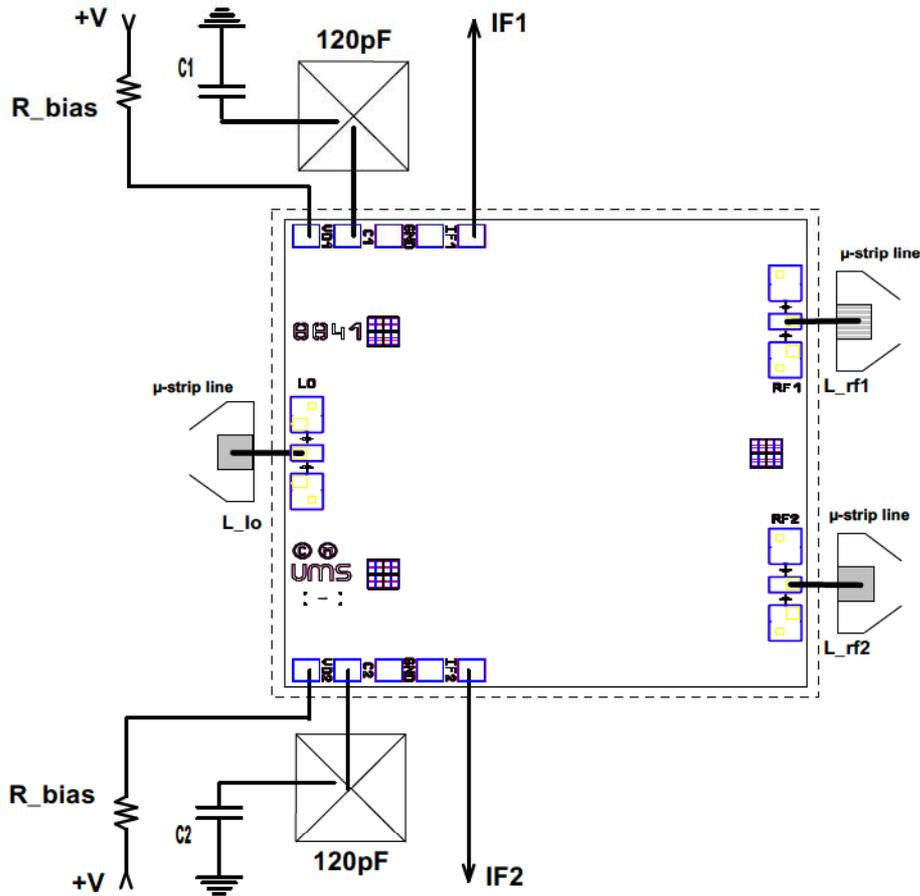
This drawing shows an example of assembly configuration. The bias and IF interconnections are according to the example given in the previous chapter. For the RF pads the equivalent wire bonding inductance (diameter=25 $\mu$ m) have to be according to the following recommendation.
